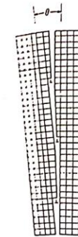
FIGURE 4-20 The small angle grain boundary is produced by an array of dislocations, causing an angular mismatch \theta between the axes on either side of the boundary.
